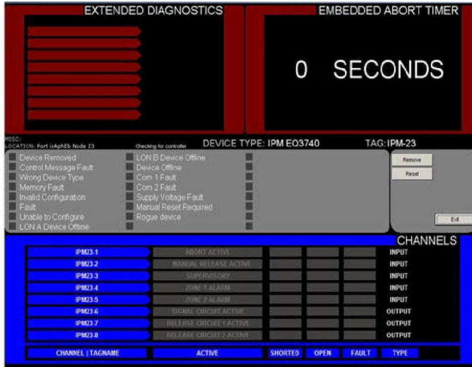
The point display provides a single window view of all available real-time data for the device. The bottom half of the point display provides a data display area and annunciator for all 8 inputs and outputs.
