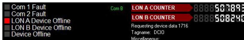
If a node on the schematic is selected (by single-clicking on its rectangle) the five indicators in the lower left of the screen will show the diagnostic data from the selected node.
