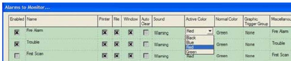
These color selections are made from the pull-down menu located to the right of the event name. The color selections apply to both printed and screen presentations of the event. In the example above, the event will be shown in Red when active and Green when it returns to normal.
