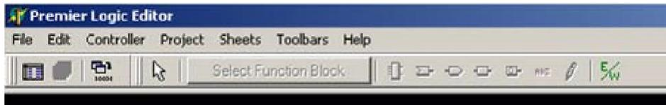
There are seven standard Windows pull down menus; File, Edit, Controller, Project, Sheets, Toolbars and Help. Each menu will be described in detail later. The button bar can be customized, but in the examples above and below, it is shown in its default configuration.
