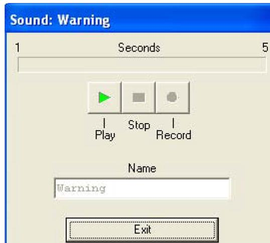
Use the "Record" button to begin recording. The horizontal bar graph will display the elapsed time. Press the "Stop" button to end the recording. Use the "Play" button to play back the recorded sound.
