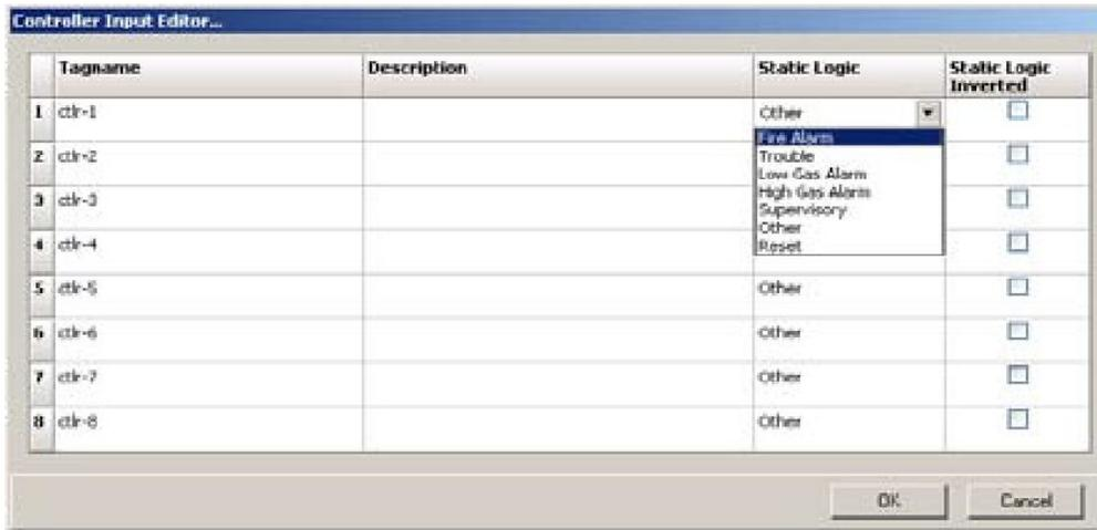
Each point can be logically “inverted” by using the checkbox in the “Static Logic Inverted” column. If the use of “Static Logic” is required, use the appropriate checkbox to enable this feature on a point-by-point basis and enter a tagname and description appropriate to the desired function(s).
