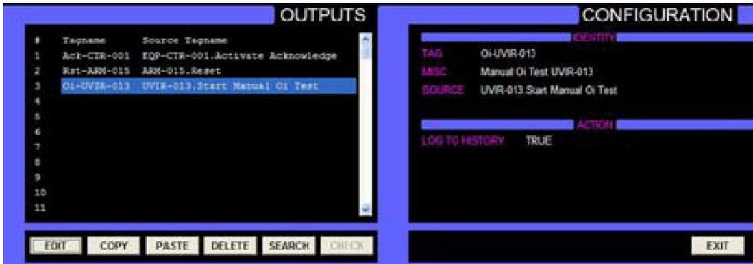
The three examples for output tags are now complete and the configuration information is displayed on the “Outputs Configuration” screen.
